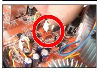
A higher fan speed will be helpful for better airflow and heat-dissipation. Nevertheless, stay alert to not touch any heatsink since a high temperature generated by the working system is still possible.
